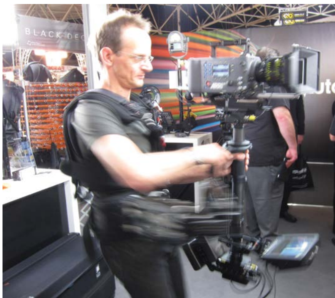
2010. Curt Schaller with ALEXA on artemis Cine HD Pro stabilizer system from Sachtler, with ACT2 Vest, artemis ACT2 Spring Arm, Transvideo CineMonitorHD 6" SBL, and Anton/Bauer Dionic-HC Li-Ion batteries.
